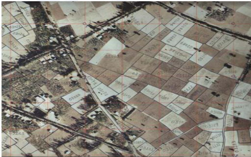
Orthophoto used as a field work map sheet with a georeferenced grid. The map shows the delineated parcel boundaries and parcel identification numbers.
