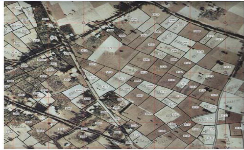
Vectorised field map showing the resulting cadastral map with parcel boundaries and cadastral numbers.
