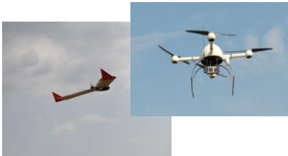
Glider/Helicopter type UAVs (150-300m, 20cm)
