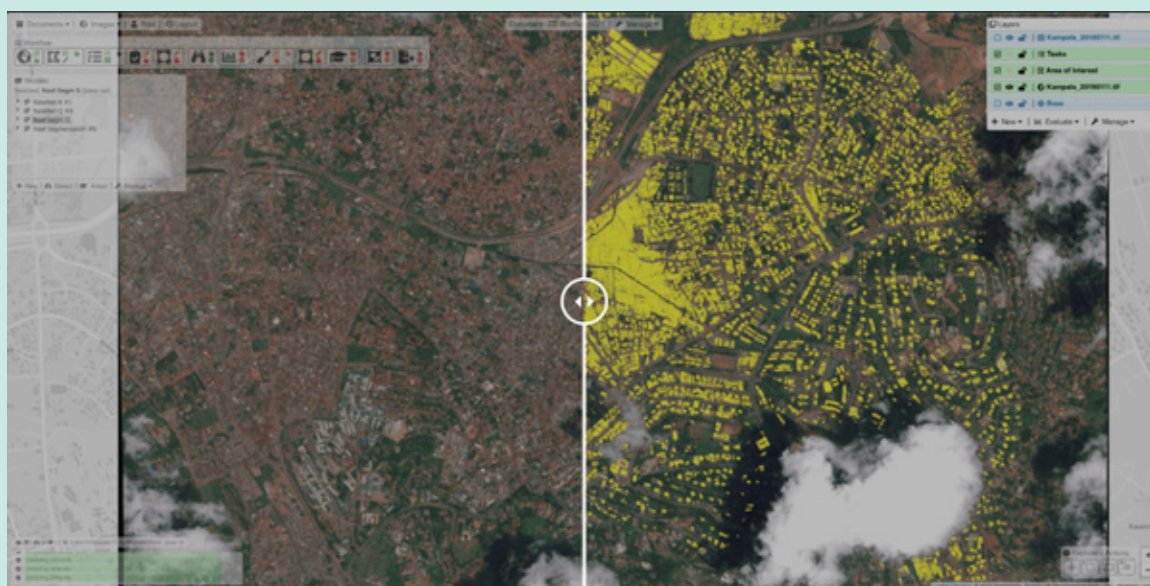
Figure 9.5 PulseSatellite's roof segmentation model used for rapid slum mapping
